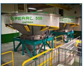
Ostara's reactors isolates nutrients from wastewater at sewage treatment plants to make fertilizer.
